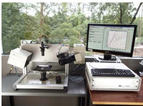
*Figure 1.* The ellipsometer in the MATinspired lab can accurately determine the thickness of thin coatings.
